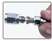
Step Three: Push the olive sleeve around the PTFE and between the braid. This can be done by pushing the olive sleeve against the side of your workbench or vise. Be sure the PTFE liner is square to the bottom of the olive. With the nipple in the vise, lube the threads and the nipple portion of the hose end sparingly. Insert the hose over the nipple making sure the olive does not pop off the PTFE tube.
