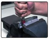
**Step Two:** Unscrew the red socket of the hose end from the nipple. Hold the socket in a vise using soft jaws and insert the hose into the socket by turning it counterclockwise. The hose will stop at the bottom step of the socket.
