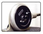
Step Five: Make sure your die number is correct for hose you are crimping. Lift handle to top position opening dies. Place end assemble in dies. Align edge of the collar (at hose) with back face of dies, using over center action push down on handle until assembly releases from crimper. Inspect assembly, be sure to wash & pressure test prior to use.
