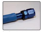
**Step Two:** Liberally oil inside of hose & barbed end of hose end. Insert barbed end into hose using a twisting action. Put the swivel end at center hex in a vise. Use a twisting motion make bottom of hex even with hose edge, rubber insulator will cover end of hose.
