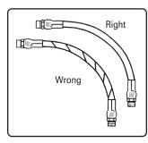
Avoid installing the hose in a twisted position.
