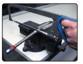
Step One: Wrap hose tightly with race or electrical tape at the point determined for cut. Clamp the hose loosely in a vise close to the tape. Use a hacksaw with two blades opposing one another or abrasive cut-off wheel. Remove the tape when you are finished cutting.
