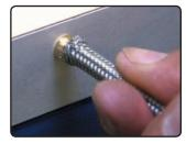
**Step Two:** Insert the nipple portion of the PowerFlex hose end in a vise. Slip the hose over the nipple using a twisting motion to size the I.D. of the Teflon. Separate the wire braid from the O.D. of the PTFE tube with a small screwdriver. Be careful not to crush the Teflon.
