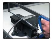
**Step One:** Wrap the hose tightly with electrical or racers tape. Hold the hose firmly in a vise without crushing and cut through the tape. Make sure you make a straight cut. Remove the tape slowly and deburr the PTFE edges. Install the socket on the hose and slide it back out of the way.
