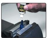
**Step Three:** Position the nipple assembly of the hose end in the vise using soft jaws. Apply assembly lube to the threads of the socket as well as to the nipple assembly.
