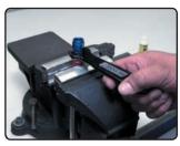
**Step Four:** Start the socket over the nipple by hand and tighten as far as possible by hand. Using an AN wrench, tighten until it reaches the nipple hex or when there is no more than 1/16" gap between the nipple/ socket assembly. Be sure to wash & pressure test the assembly before using.
